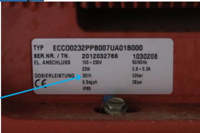
Close up of the name plate of an individual feed pump. Dosierleistung is translated as dosing capacity or maximum flow.
